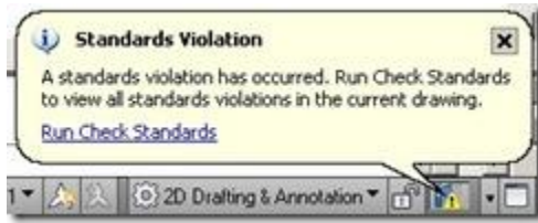
Figure 19 - Standard violation warning
